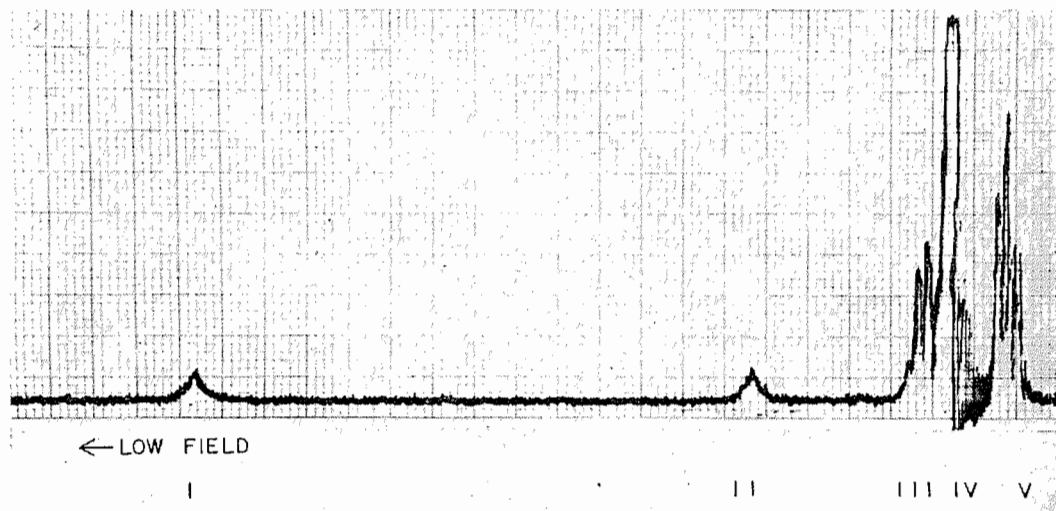
FIG. 8. PMR spectrum of acetylacetone in triethylamine, mole fraction 0.66. Assignment of signals: I, enol —OH; II, enol —CH=; III, triethylamine, —CH 2 —; IV, enol methyl; and V, triethylamine CH 3 —.
